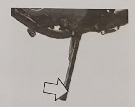
To use the main, depress it by foot and lift the rear of the motorcycle until the rear wheel is lift. To use the side, depress the end of it until it rotates to the end and stops.
