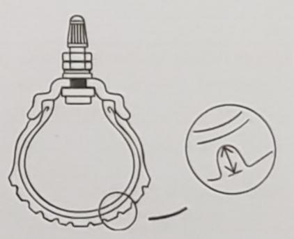
Operating the motorcycle with excessively worn tyres will decrease riding stability and can lead to loss of control. It is recommended that a tyre be replaced when the remaining depth of tyre tread becomes 1.6mm or less.
