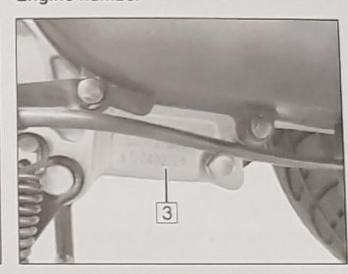
The engine number (3) is located on the front part the left crankcase.
